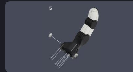
Add two 4mm bearings and pop the joint in
