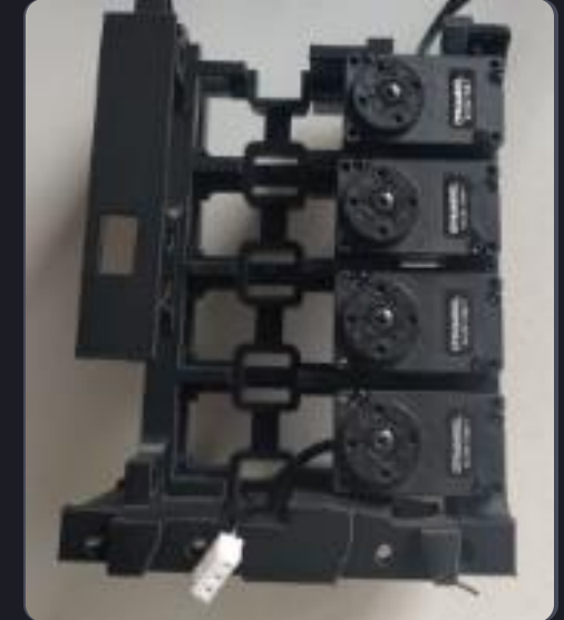
Assemble the motors onto the tower
