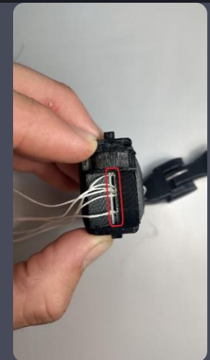
Insert two 2×30 pins, tendons seated between them, order kept
